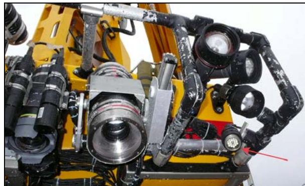
Figure 4. Canadian Scientific Submersible Facility - ROPOS ROV before an evaluation dive with DSPL's 2000-lm LED-MultiSeaLite ® (red arrow), and other lights. Photo by Reuban Mills, ROPOS
