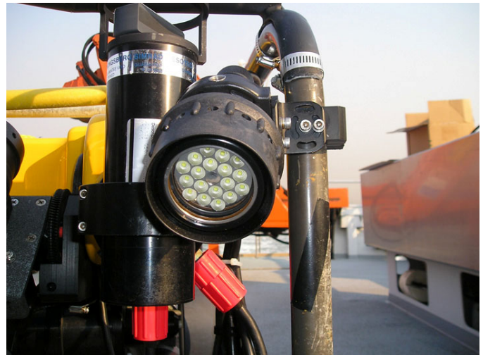
Figure 3. A DeepSea Power & Light LED Multi-SeaLite® illuminates the field-of-view for Los Angeles County's Phantom ROV.
