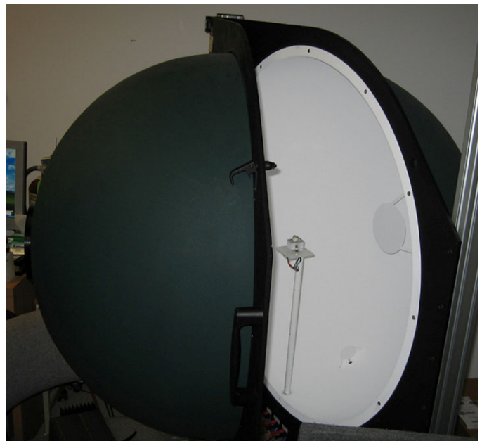
Figure 2. An Integrating Sphere provides a precise and repeatable measurement of total light and color emitted from a lamp.
