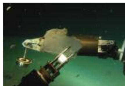
*Piece of hard gas hydrate in the manipulator of the MIR*
