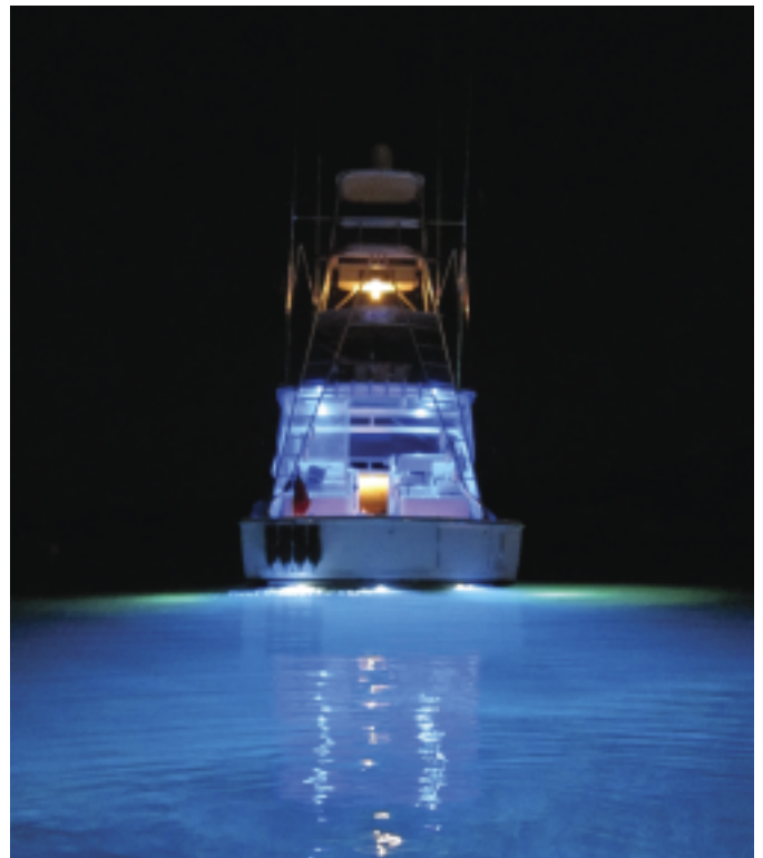
Because of their excellent vibration resistance and long life, underwater LED lights are also used for thru-hull applications on recreational boats. This 36-ft. Cabo sportfishing boat has three white, three blue, and three green 12-LED On-Hull SeaLites® mounted below the water line in its transom as well as one white 18-LED Thru-Hull SeaLite mounted on each side
