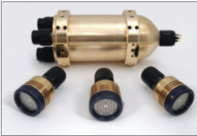
An advanced remote head system configuration with three remote LED light heads and a single ballast housing containing the drivers for all remote heads. Housing material in this case is beryllium copper for use in a special long-term immersion application
