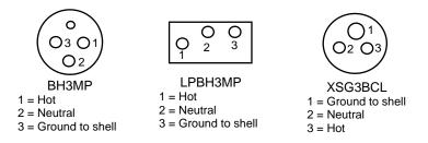
Figure 1: Standard Deep-SeaLite® Connector Pinouts
