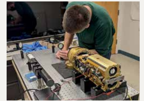
» The MxD SeaCam chassis optical block and lens are precision aligned with the adapter cell using laser reflections from each lens surface. An MBARI engineer sets up the alignment test on an optical bench. (Photo credit: Mark Chaffey © 2021 MBARI)
