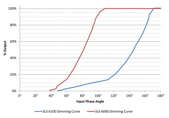
**SLS-6100 Variable Voltage Dimming Response**
