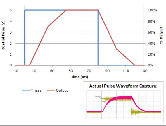
Low-Voltage DC Step Response Curve for both SLS-3100 & SLS-5100
