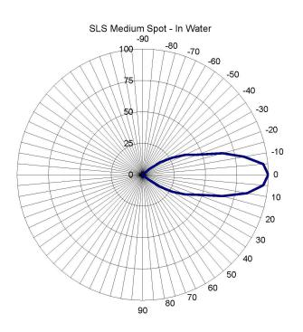
SeaLite Sphere Beam Pattern SLS Medium Spot - In Water
